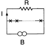
Fig. 1. Circuit schematic of a Josephson junction series array, subject to a parallel resistive load. Each cross represents a Josephson element.
