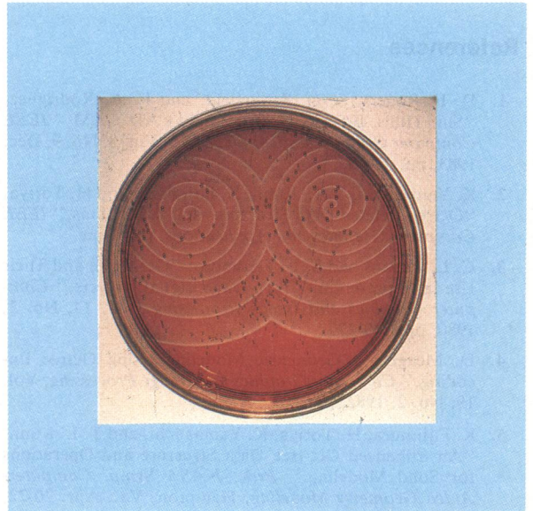
Figure 1. Colored waves of chemical activity move like expanding mirror-image spirals in a thin film of the Belousov-Zhabotinsky reagent. (Photographed in the laboratory of Arthur T. Winfree by F. Goro for Scientific American . 2 )
